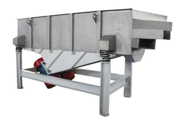
RECTANGULAR VIBRATING SIEVE adopt vibrating motor excitation as the vibration source, Two vibration motors installed on the equipment which work in simultaneously (Vibration develop in the horizontal and in the vertical plane).
