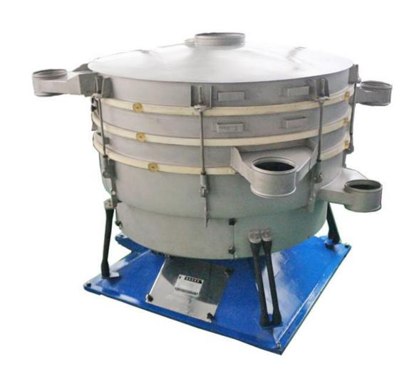
Dingcoma tumbler screening separator is used for control screening, fractionating and dust removal in dry, powdered and granular products. The tumbler screening machine has a three dimensional movement similar to the simple hand screening of the "gold washing pan". This tumbline action yeilds better efficiency and a higher specific screen load as compared to vibration systems.
