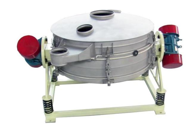
Direct discharge vibrating screen is the two models of the same vibration motor mounted symmetrically on both sides of the screening machine, the vibration motor and lower ends are equipped with eccentric weights, generated during rotation of the horizontal, vertical, inclined three-dimensional movement
